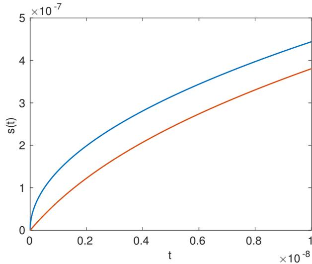
Figure 2: Evolution of the solid-liquid interface. The physical parameters used correspond to Silicon. The red line is the solution to the model with varying thermal conductivity and the blue line to the problem with bulk thermal conductivity.
